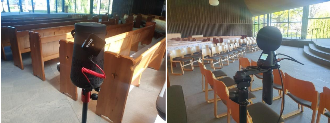
Figure 4: IRIS Mini kit Bose Soundlink Revolve+ II speaker source (left) and Zoom H3-VR receiver (right)
