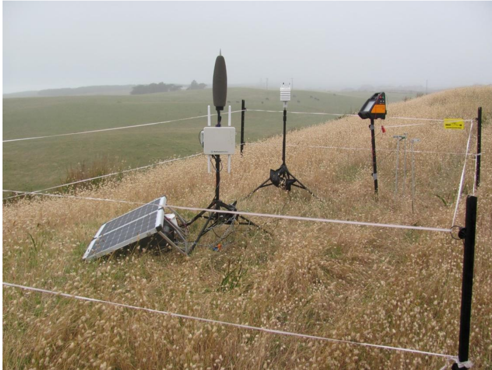
Figure 2: Typical noise monitoring system
